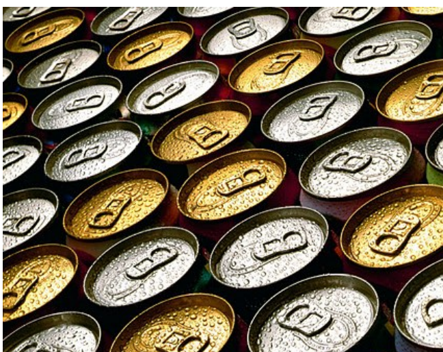
Aluminium cans, which dominate the beverage cans' market consists of about 2.5% magnesium 鋁罐主導了飲料罐的市場含有約2.5%的鎂金屬
