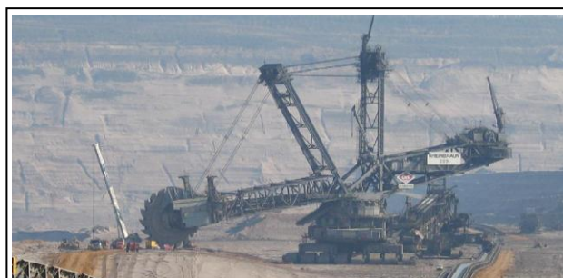
Bucket wheel excavator used in open pit mining 用於露天開採的旋轉輪挖礦車
